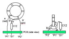
Diagram showing logical connection (on left), and physical connection (on right) for T1
